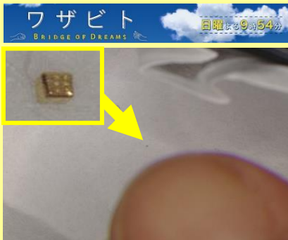
Successful plating on dice of 100 \mu m.
